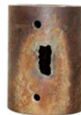
4-1/2" 15.1# Tubing Circulating Pyro Torch® cut @ 20,000psi
