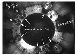
A deep-water operator in the Gulf of Mexico sought to ensure there was no debris on the shoulder of the sensor and control stabs in the tubing hanger of this subsea wellhead. Any debris could damage the stabs during the latch up which would require pulling the entire completion for repair. The image shows the shoulder free of debris and was used to align the connection before latching.
