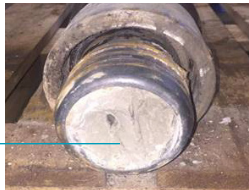
Cement sample recovered from beneath the latch in adapter ball seat of the SeaCure® system. A qualitative but definitive example of cement quality at the shoe.
