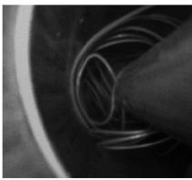
Top of the tool rope socket covered by metal particles; also the images of the wire coiled across the tool confirming the rope socket (tool head) is free from any exposed wires
