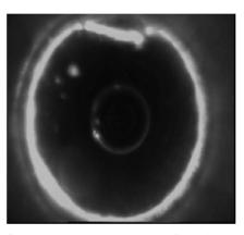
Damage can be seen on the top flow tube of the TRSCSSV and the same image seen on impression of the 3.75" LIB
