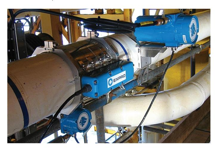
We utilise clamp-on sonar-based meters and innovative multiphase flow interpretation techniques to provide accurate and reliable flow measurement with no process interruption.
